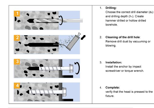
Remark : cleaning of borehole is not necessary when using an hollow drill bit
